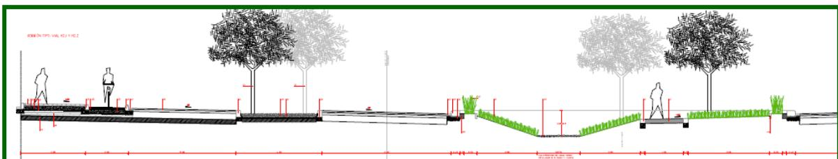
Figure 4: Cross section of the main road, integrating a current runoff corridor into the site layout
