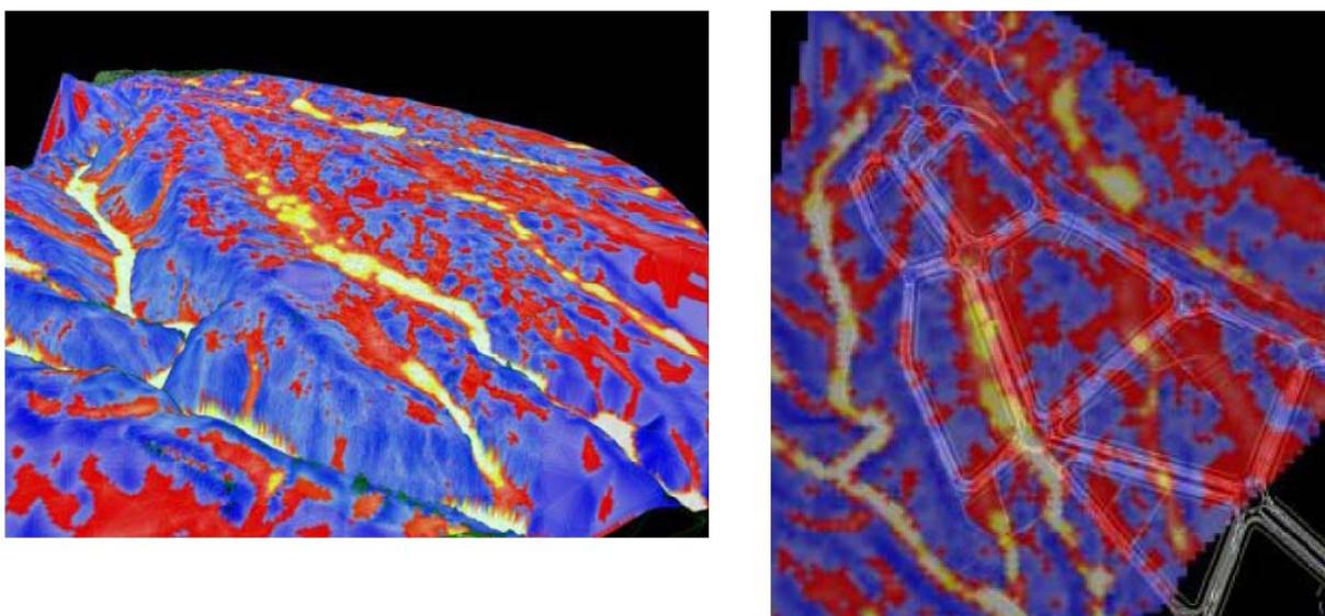
Figure 2: Natural Hydrology for Phase 1 of the Soterranyes Industrial Development, and site layout accommodating water corridors into the main roads and plot distribution
